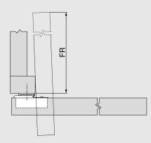
Hinge dimensions and gap calculation based on factory setting \* prevent collision
